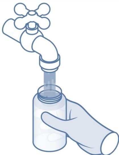
2. **Fill the sample bottle** to the shoulder or the line marked “250 ml”. Close the cap tightly.
