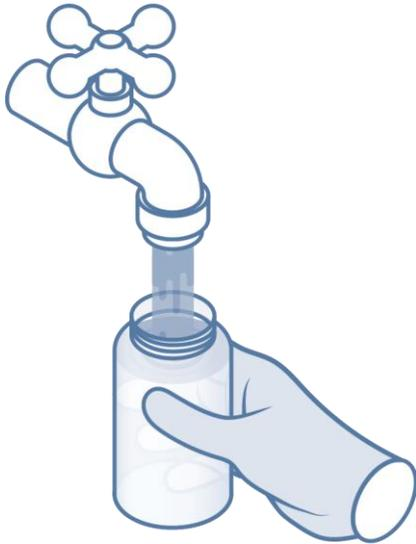
2. **After 30 seconds**, while the water is flowing place the sample bottle under the fixture and fill the sample bottle to the shoulder or the line marked “250 mL”. Close the cap tightly.
