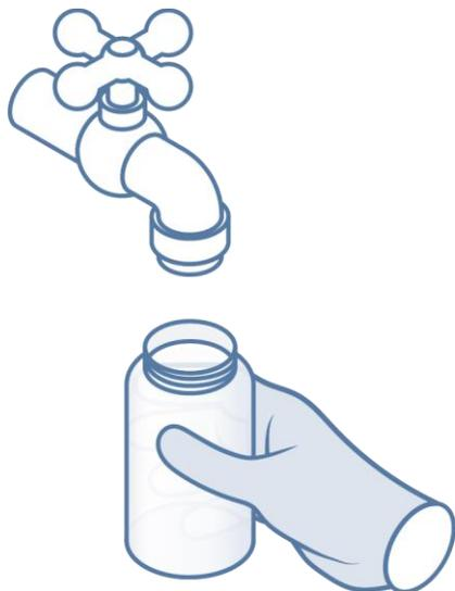
1. **First thing in the morning**, place the sample bottle under the fixture and open the cold water tap to a normal flow.
